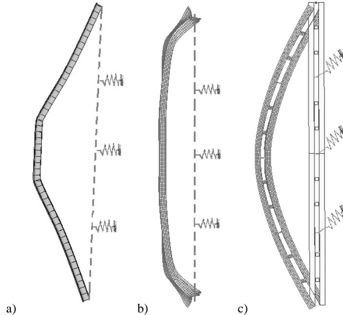
Fig. 6. Deformation of the bar at the limit state for supports stiffness  $k = 1000 \text{ kN/m}$ :
