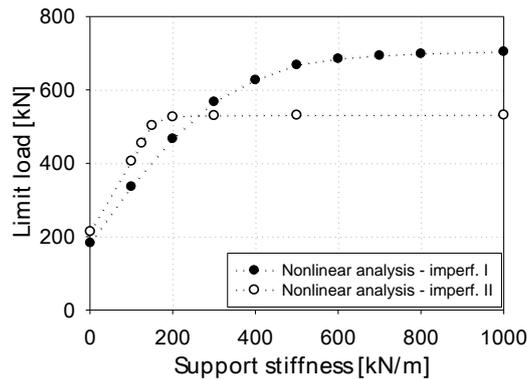
Fig. 5. The relation between the limit load for the beam model of the bar with respect to the supports stiffness (imperfection I - initial deformation perpendicular to  $y$ - $y$  axis, imperfection II - initial deformation perpendicular to  $z$ - $z$  axis)
