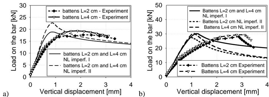
Fig. 9. The bar loading vs. vertical displacement (measured at the loaded point) for shell model and support stiffness: a)  $k = 10$  kN/m, b)  $k = 80$  kN/m. (Imperf. I - deformation perpendicular to  $y$ - $y$  axis, Imperf. II - initial deformation perpendicular to  $z$ - $z$  axis)
