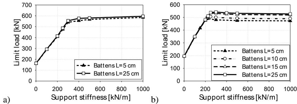
Fig. 4. The relation between the limit load for the shell model of the bar with respect to the supports stiffness: a) model with imperfection I (shape of imperfection - deformation perpendicular to  $y$ - $y$  axis), b) model with imperfection II (shape of imperfection - deformation perpendicular to  $z$ - $z$  axis)
