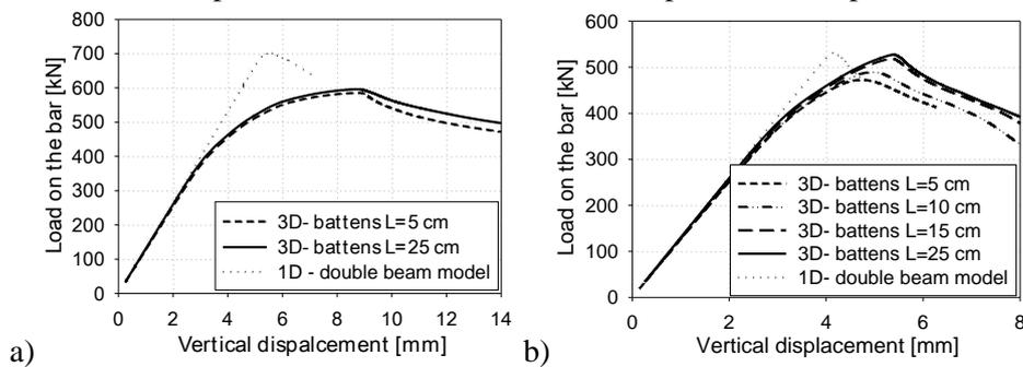
Fig. 3. The bar loading vs. vertical displacement (measured at the loaded point) for beam and shell model with: a) imperfection I (shape of imperfection - deformation perpendicular to  $y$ - $y$  axis), b) imperfection II (shape of imperfection - deformation perpendicular to  $z$ - $z$  axis)
