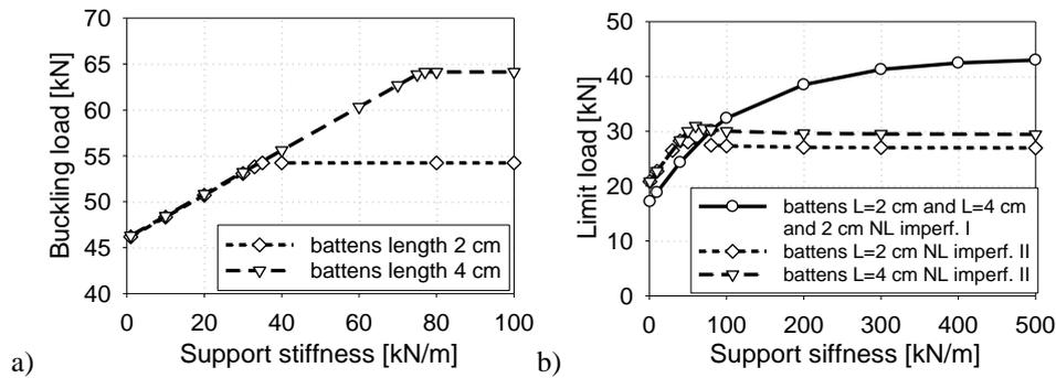
Fig. 8. The relation between: a) buckling load, b) limit load - with respect to the support stiffness, for the shell model of the structure tested experimentally
