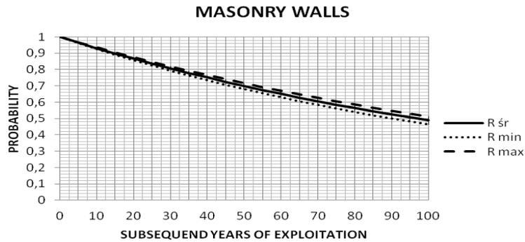
Fig. 1. Reliability prediction of masonry walls according to the exponential distribution
