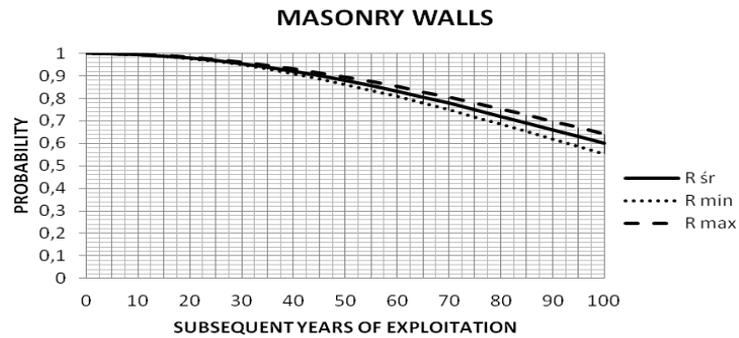
Fig. 2. Reliability prediction of masonry walls according to the Rayleigh distribution
