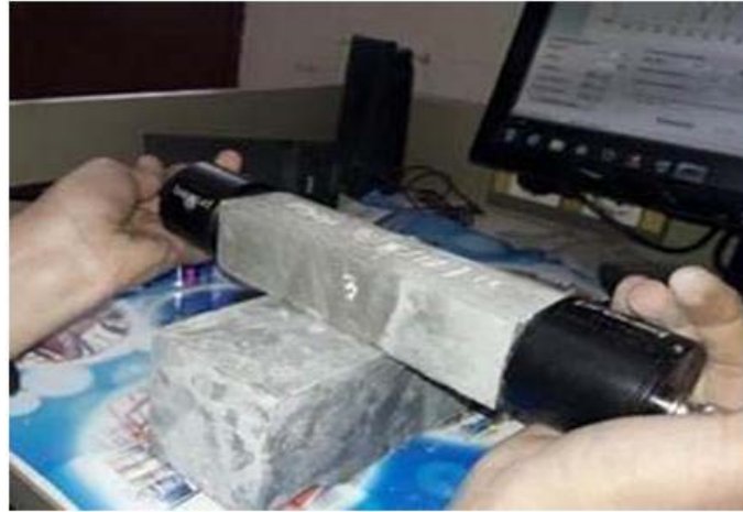
Fig.6. Ultrasonic pulse velocity tests carried out on prismatic samples.
