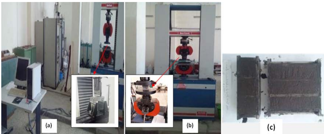
Fig.5. Mechanical testing: (a) flexural tests, (b) compressive and behavior mechanical, (c) cubic and prismatic specimens.
