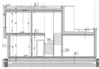
Fig. 4a. Two-storey house in Pilchowice, cross section; authors' own illustrations
