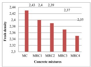
Fig. 4. Fresh density values of concrete mixtures
