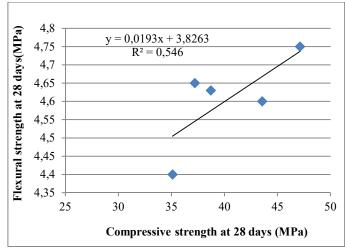
Fig. 8. Relationship between Compressive strength and flexural strength
