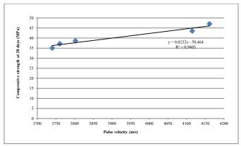
Fig. 10. Relationship between Compressive strength and pulse velocity
