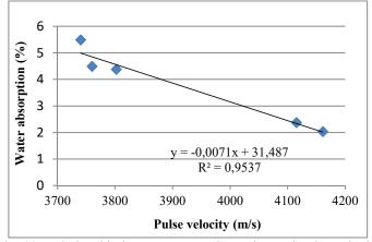
Fig. 12. Relationship between water absorption and pulse velocity
