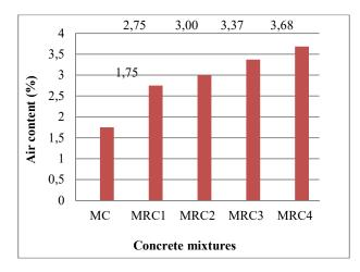
Fig. 5. Air content values of concrete mixtures
