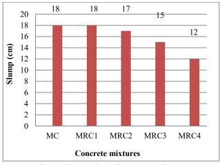
Fig. 3. Slump values of concrete mixtures
