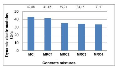
Fig. 14. Dynamic elastic modulus values of concrete mixtures
