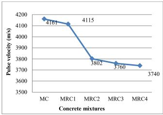
Fig. 9. Pulse velocity values of concrete mixtures
