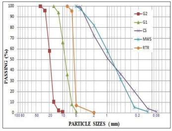
Fig. 2. Particles size distribution of aggregates
