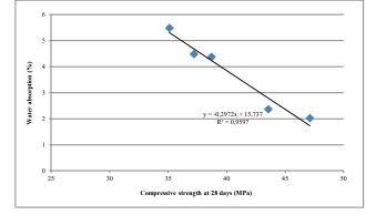
Fig. 13. Relationship between water absorption and compressive strength
