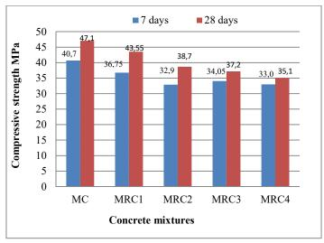
Fig. 6. Compressive strength values of concrete mixtures
