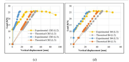
Fig. 7. Comparison of experimental verticals displacement with theoretical results: c) Beam CB3, d) Beam B4
