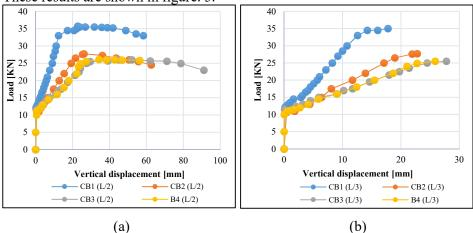
Fig. 5. Variations in vertical displacement as a function of transverse load: a) Vertical displacement (L/2), b) Vertical displacement (L/3)
