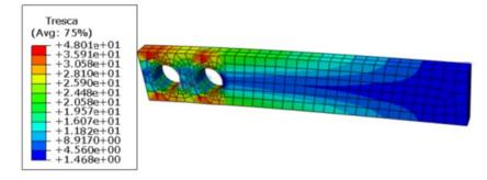
Fig. 11. FE model for beam with circular cuts in their webs
