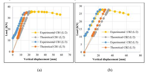
Fig. 6. Comparison of experimental verticals displacement with theoretical results: a) Beam CB1, b) Beam CB2
