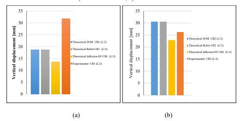
Fig. 9. Comparison of the maximum experimental vertical displacement of beams with the maximum theoretical vertical displacement from the SOM, Robot structures and Inflexion-EF programs: a) CB1, b) CB2
