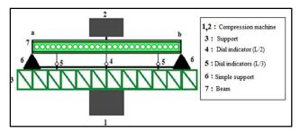
Fig. 3. Test device
