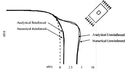
Fig.8. Stress distribution along of the hole edge in  $(0)_{12}$  laminate sequence for a reinforced hole for a stress ratio of SCF.
