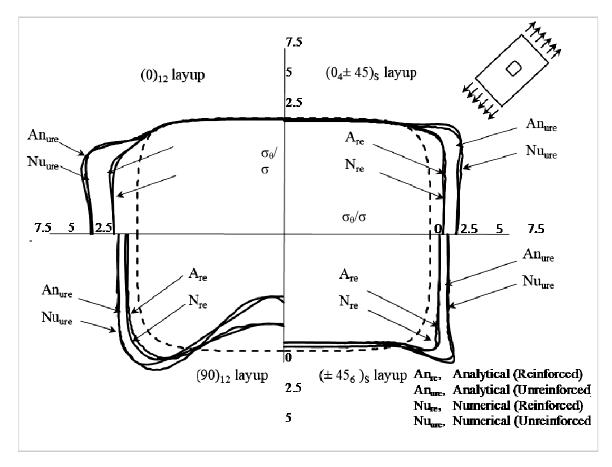
Fig.5. Stress distribution along of the hole edge in  $(0)_{12}$ ,  $(0_4 \pm 45)_S$ ,  $(\pm 45_6)_S$  and  $(90)_{12}$  laminate sequence for an unreinforced and reinforced hole.
