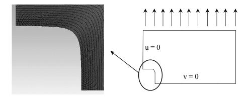
Fig.2. Finite Element Model of the plate.
