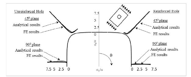
Fig.7. Stress distribution ahead of the hole edge in  $(\pm 45_6)_S$  laminate sequence for a unreinforced and reinforced hole.
