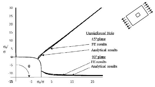
Fig.6. Full field stress distribution in  $(0)_{12}$  laminate sequence.
