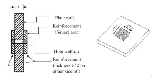
Fig.1. Reinforcement scheme.
