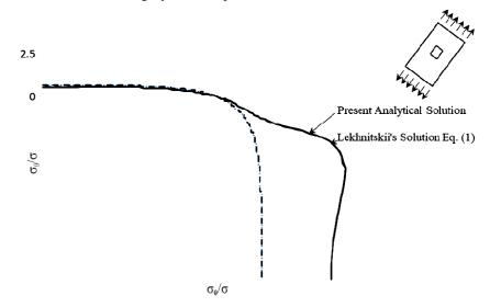
Fig.3. Comparison of stress distribution along the hole edge obtained by the present analytical solution andLekhnitskii's solution.
