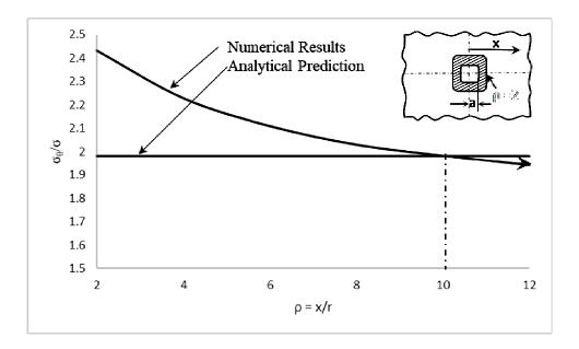
Fig.4. Comparison of maximum SCF along a reinforced square hole edge for various area of reinforcement obtained from analytical and numerical model.
