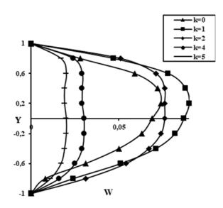
Fig.9 Secondary velocity for different K and  $H_a = 10$ ,  $\alpha = 0.333$ ,  $\sigma_0 = 2$ , m = 2,  $\sigma_1 = 1.2$ ,  $\rho = 1$ ,  $\sigma_2 = 1.5$ , h = 0.8.
