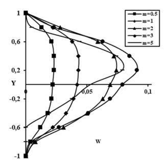
Fig.6. Secondary velocity for different *m* and  $\alpha = 0.333$ ,  $H_a = 10$ ,  $\sigma_0 = 2$ , K = 2,  $\sigma_1 = 1.2$ , h = 0.3,  $\sigma_2 = 1.5$ ,  $\rho = 1$ .
