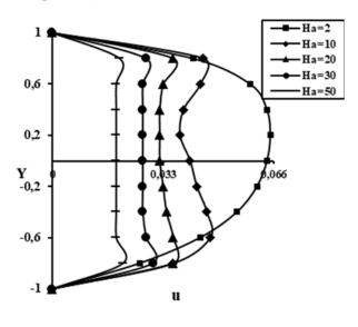
Fig.2. Primary velocity for different  $H_a$  and  $\alpha = 0.333$ ,  $\sigma_0 = 2$ , h = 0.8,  $\sigma_1 = 1.2$ , m = 2,  $\sigma_2 = 1.5$ , K = 2,  $\rho = 1$ .
