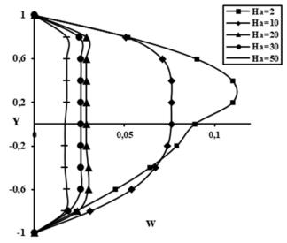
Fig.3 Secondary velocity for different  $H_a$  and  $\alpha = 0.333$ ,  $\sigma_0 = 2$ , h = 0.8,  $\sigma_1 = 1.2$ , m = 2,  $\sigma_2 = 1.5$ , K = 2,  $\rho = 1$ .
