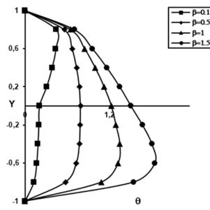
Fig.17. Temperature for different  $\beta$  and  $H_a = 10, h = 0.8, \alpha = 0.333, s_0 = 2, m = 2,$  $s_1 = 1.2, s_2 = 1.5, K = 2, \rho = 1.$
