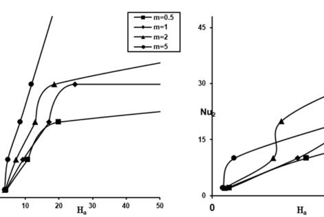
Fig.18. Nusselt number  $Nu_1$  for different  $H_a$  and a = 0.333, h = 0.8,  $s_0 = 2$ , K = 2,  $s_1 = 1.2$ ,  $s_2 = 1.5$ ,  $\rho = 1$ , b = 1.
