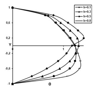
Fig.16. Temperature for different *h* and a = 0.333,  $H_a = 10$ ,  $s_0 = 2$ , K = 2,  $s_1 = 1.2$ ,  $s_2 = 1.5$ , m = 2, r = 1, b = 1.
