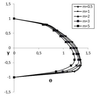
Fig.7. Temperature for different *m* and  $H_a = 10$ , h = 0.8,  $\sigma_0 = 2$ , K = 2,  $\sigma_1 = 1.2$ ,  $\sigma_2 = 1.5$ ,  $\rho = 1$ ,  $\beta = 1$ ,  $\alpha = 0.333$ .
