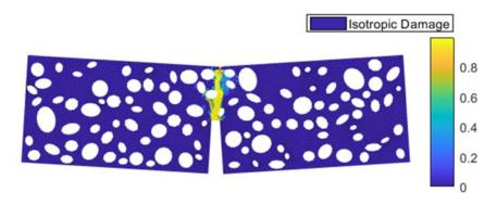
Fig.8c. Crack propagation of realization 20 (maginification factor is 20): CMOD=0.3032mm.
