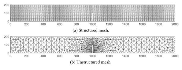
Fig.1. Structured and unstructured mesh.
