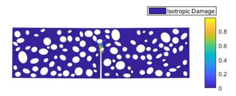
Fig.8a. Crack propagation of realization 20 (maginification factor is 20): CMOD=0.02558mm.
