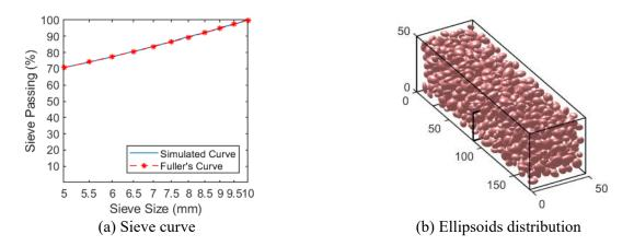
Fig.4. Sieve anlysis and ellipsoids distributions.
