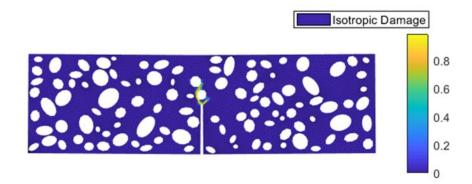
Fig.7a. Crack propagation of realization 3 (maginification factor is 20): CMOD = 0.02545 mm.
