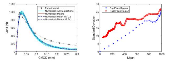
(a) Load-CMOD curves (b) Mean vs. standard deviation of numerical results Fig.6. Load-CMOD curves of experimental data and numerical models.
