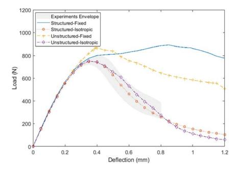
Fig.2. Load-deflection curves of experimental data and numerical models.
