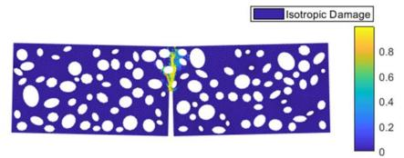
Fig.8b. Crack propagation of realization 20 (maginification factor is 20): CMOD=0.1064mm.
