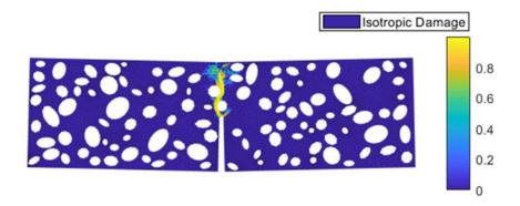
Fig.7b. Crack propagation of realization 3 (maginification factor is 20): CMOD=0.1047mm.
