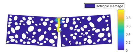
Fig.7c. Crack propagation of realization 3 (maginification factor is 20): CMOD=0.3021mm.
