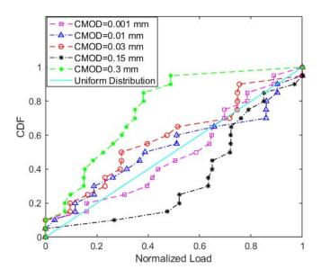
Fig.10. The variation of CDF for different CMOD values using 20 realizations.
