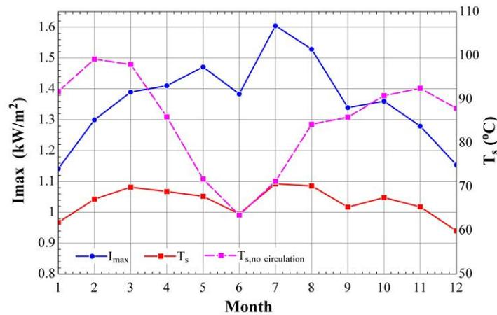
Fig. 2. Peak solar irradiance ( $I_{max}$ ), solar cell temperature with cooling ( $T_s$ ) and solar cell stagnation temperature ( $T_s$ , no circulation) at peak irradiance for each month of operation
