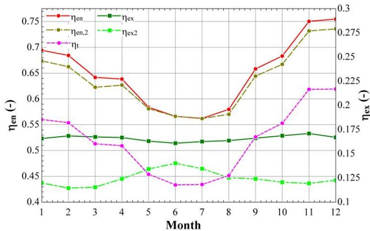
Fig. 6. Thermal efficiency of the PV/T collector ( $\eta_t$ ), 1<sup>st</sup> ( $\eta_{en}$ ) and 2<sup>nd</sup> ( $\eta_{ex}$ ) efficiencies of the PV/T+ORC system and of the PV/T system with no circulation of fluid ( $\eta_{en,2}$ ,  $\eta_{ex,2}$ ) at peak irradiance
