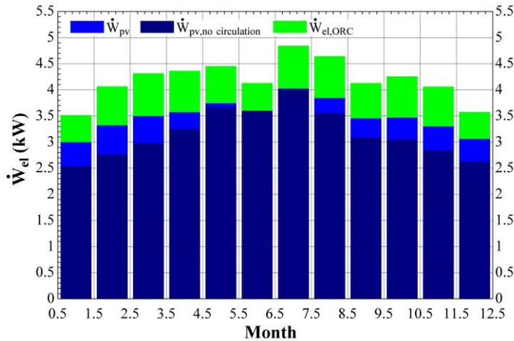
Fig. 5. Electric power generated by the PV cells with ( $\dot{W}_{PV}$ ), without circulation of fluid ( $\dot{W}_{PV, no\ circulation}$ ) and total electric power generated by the PV/T+ORC system ( $\dot{W}_{el, ORC}$ ) at peak irradiance for each month of operation
