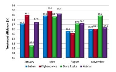
Fig. 2. Efficiency of COD removal
