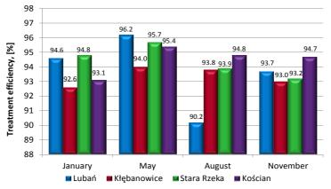
Fig. 3. Efficiency of removing the total suspension solids
