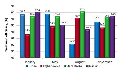
Fig. 1. Efficiency of BOD<sub>5</sub> removal
