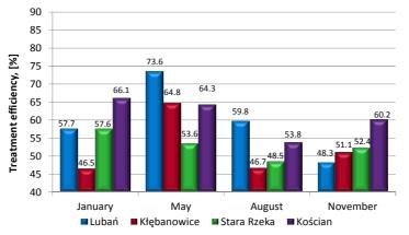
Fig. 5. Efficiency of total phosphorus removal
