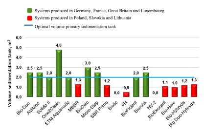
Fig. 2. Primary sedimentation tank volume in the analysed wastewater treatment systems
