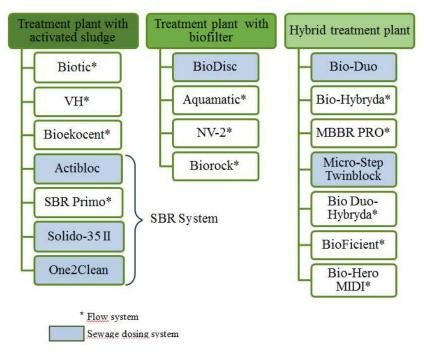
Fig.1. Technologies of individual sewage treatment systems
