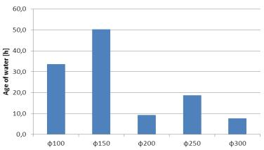
Fig. 6. Values of weighted averages of the age of water for individual pipeline diameters in Lubin
