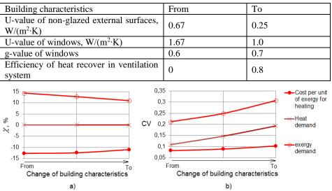
Fig. 4. Values of deviation betweeen dynamic and steady state approach for annual energy/exergy parameters and of coefficient of variation with different building characteristics
