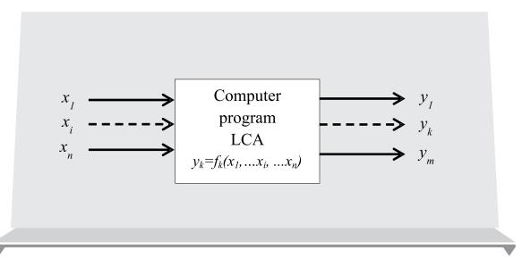
Figure 1. The scheme of life cycle assessment (LCAa) with the use of a specialized computer program: xi = input signals; i = 1 ... n where n = number of input signals; yk – output; k = 1 ... m where m = number of output signals
