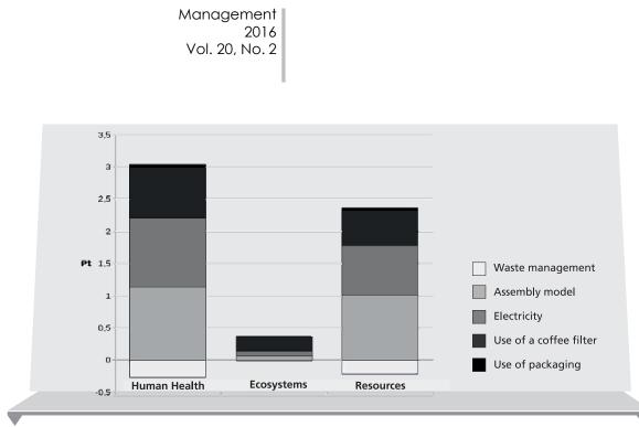
Figure 4. Life cycle impact assessment of the coffee machine model SimaPro in the endpoint impact categories
