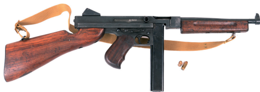
Pistolet maszynowy Thompson 1928 M1A1, kal. 11,43 mm (Auto-Ordnance, Bridgeport, CT)
