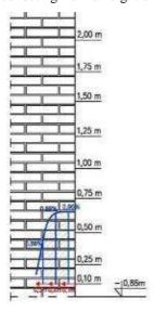
Fig. 10. Sulphates salinity distribution graph at a depth of 0.1; 0.2; 0.3 masonry structural wall from the inside at the samples collecting from a height of 0,1m
