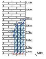
Fig. 5. Sulphates salinity distribution graph at the height of masonry basement walls at the samples collecting from depths of 0,1m
