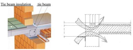
Fig. 4. Thermal bridges at the connection of the floor with a cantilevered balcony. The corners where the floor-wall meets lose heat (freezing effect - the occurrence of mold and mildew)
