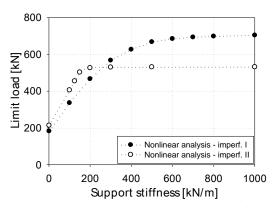
Fig. 5. The relation between the limit load for the beam model of the bar with respect to the supports stiffness (imperfection I - initial deformation perpendicular to *y*-*y* axis, imperfection II - initial deformation perpendicular to *z*-*z* axis)
