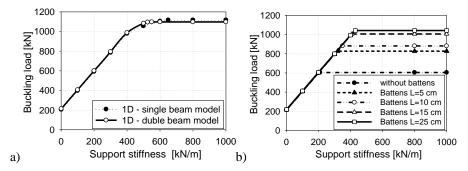
Fig. 2. The relation between the first buckling load for the bar with respect to the supports stiffness: a) beam model, b) shell model
