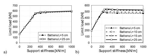
Fig. 4. The relation between the limit load for the shell model of the bar with respect to the supports stiffness: a) model with imperfection I (shape of imperfection - deformation perpendicular to *y*-*y* axis), b) model with imperfection II (shape of imperfection - deformation perpendicular to *z*-*z* axis)
