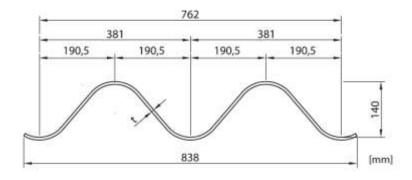
Fig. 6. Cross-section the SuperCor
