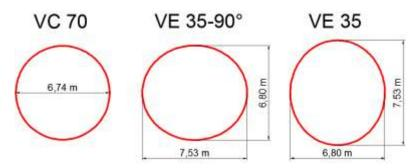
Fig. 8. Shapes and general dimensions of compared shells
