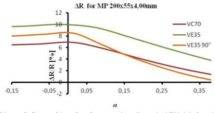
Diagram 7. Change of the radius of curvature depending on backfill height for a shell of  $4,00~\mathrm{mm}$  thickness
