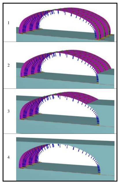
Fig. 7. Selected stages of backfilling
