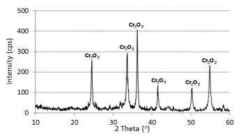
Fig. 5. XRD pattern of residue ash
