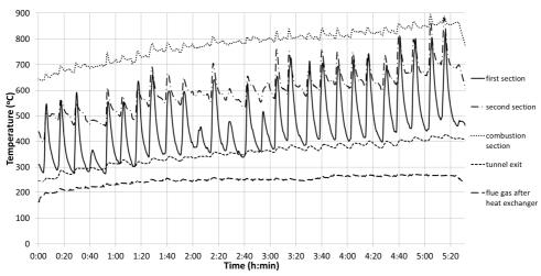
Fig. 3. Furnace temperature vs. time diagram
