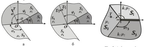
Fig. 2. The scheme of a system loaded by internal concentrated force
