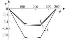
Fig. 4. The function of distribution of the tangential stresses  $\tau$  under conditions of the first boundary-value problem
