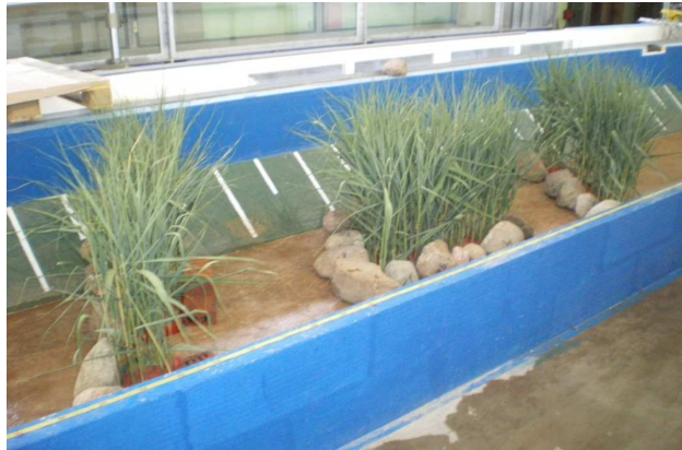
Fig. 6. Laboratory model of fishway with biotechnical build-up
