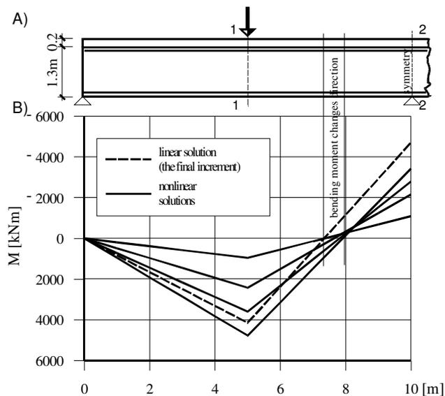
Fig.7.A) Structural system. B) Bending moments in the girder. Comparison of the linear and the nonlinear solutions in some subsequent increments of the load
