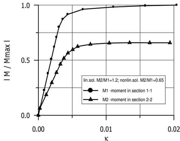
Rys. 8. Bending moment – curvature relations in sections 1-1 and 2-2
