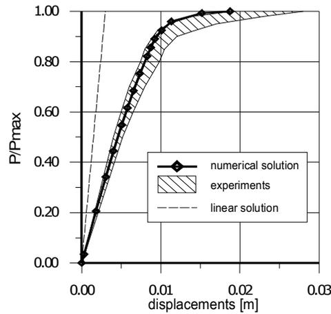
Fig.6. Deflection of the centre of the girder (section  $\alpha-\alpha$ , node 31)
