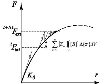
Fig.4. A modified Newton-Raphson method for one degree of freedom system
