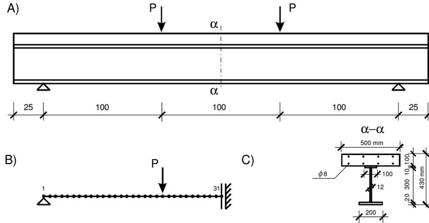
Fig. 5. A) Diagram of a composite girder, B) Division into finite elements, C) a cross section of the girder and the reinforcement of the slab
