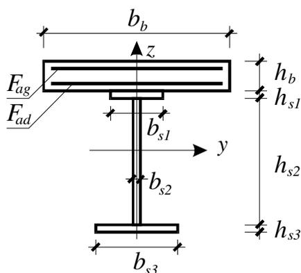
Fig.1. Cross section of a composite girder
