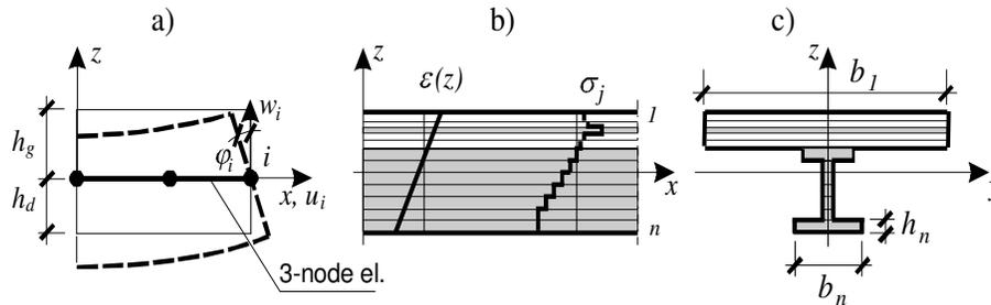
Fig.2. An element of a composite girder: a) degrees of freedom in node  $i$ , b) strains and stresses in layers, c) cross section of the element
