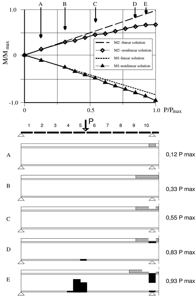
Fig.9. Bending moments redistribution and phases of girder degradation
